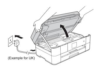
Connect the power cord. Lift the scanner cover.
