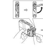
Follow the Touchscreen instructions to install the ink cartridges. The machine will prepare the ink tube system for printing.
