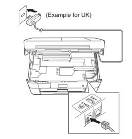
Connect the telephone line cord. Use the socket marked LINE and guide the cord out the back of the machine.
