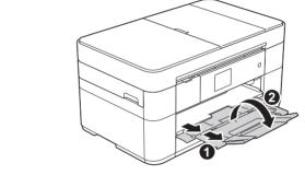
Pull out the paper support 1, and unfold the paper support flap 2.
