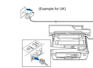
Connect the telephone line cord. Use the socket marked LINE and guide the cord out the back of the machine.
