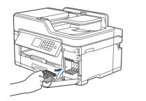
Open the ink cartridge cover, and then remove the orange protective part from the machine.
