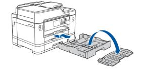
Pull the paper tray completely out of the machine as shown by the arrow. Take off the tray top cover.
