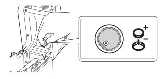
5 Return the time/date battery cover to its original position, and then use a coin or similar object to slowly turn the time/date battery cover in the opposite direction of the arrow on the battery cover until it stops in order to install the time/date battery cover.
