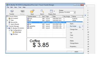
The data registered with keys 1 to 28 (1) of the one-touch panel is determined by the key number.
