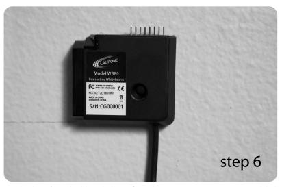
Remove backing from double-sided tape from the (1) USB corner sensor piece (labeled "R-B") and mount to the bottom right hand corner to begin the build onto the level line created in Step 3.
