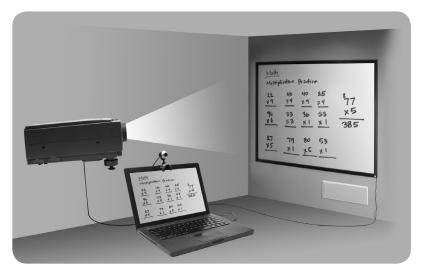
Connect a projector to the PC and align the video from the projector to display within the interactive whiteboard space.
