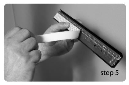
Apply all pre-cut strips of (0.5") double-sided mounting tape to Sensors
