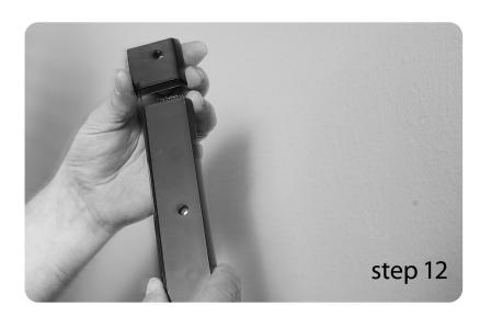
Attach corner sensor "R-U" to half-sized Sensor 4.
