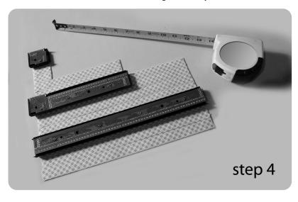
Pre-cut strips of (0.5") double-sided mounting tape into the following lengths:
