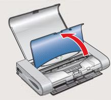
2 Press in on the lock button and lift the gray lock lever.
