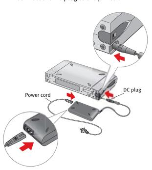
3 Plug the power cord into the power outlet.
