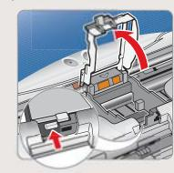
3 Remove the print head from its package. Turn the print head over and remove the protective cap from the print head cover.
