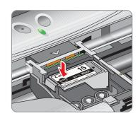
**5** Using the procedure above, insert the color ink tank into the front slot.
