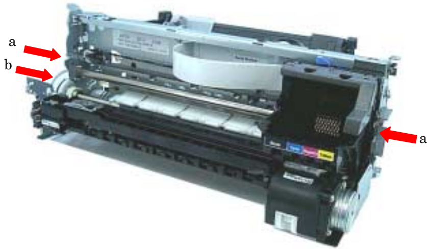
Figure 1-3 Do Not Loosen or Remove Red Screws
