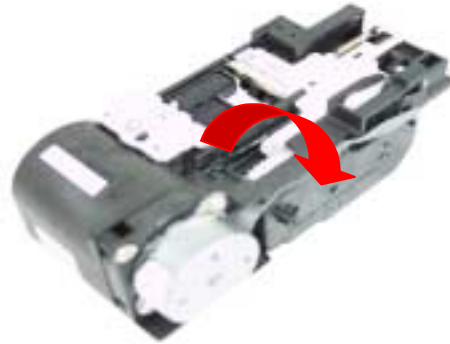
Figure 1-1 Releasing Carriage Lock
