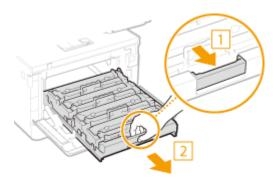
**3** Pull the target toner cartridge straight up and out of the machine.
