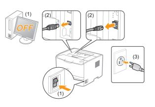
When installing or removing the optional accessories, be sure to turn the printer OFF, unplug the power plug, and then disconnect all the interface cables and power cord from the printer. Otherwise, the power cord or interface cables may be damaged, resulting in a fire or electrical shock.
