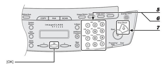
**5** Enter the destination name (max. 20 characters, including spaces) with the numeric keys, then press [OK].
