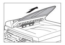
**11** Fold the paper stopper, and then push the output tray extension into the machine.
