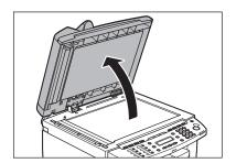
Clean the ADF scanning area (on the left side of the platen glass) and the document feeding roller with a cloth dampened with water. Then wipe the area with a soft, dry cloth.
