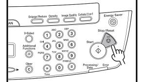
Press [Stop/Reset] to return to the standby display.
