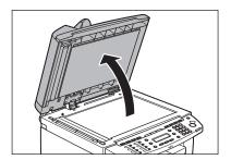
Clean the platen glass and the underside of the ADF with a cloth dampened with water. Then, wipe the area with a soft, dry cloth.
