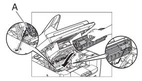
**7** Push the toner cartridge to make sure it is properly set in the machine.
