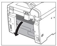
Lift the scanning platform until it is locked (A), and open the printer cover (B).
