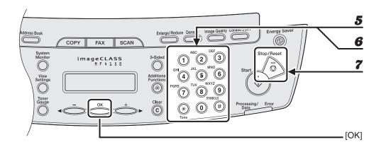
**5** Enter the destination name (max. 20 characters, including spaces) with the numeric keys, then press [OK].
