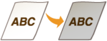
Blank space of originals becomes grayish in printouts
