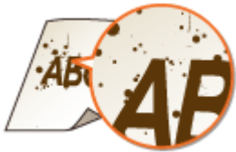
Toner smudges and splatters appear
