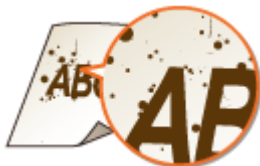
Toner smudges and splatters appear
