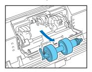
**4.** Remove any dirt from the roller using a cloth that has been soaked in water and thoroughly wrung out.
