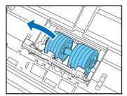
**3.** Remove any dirt from the roller using a cloth that has been soaked in water and thoroughly wrung out.
