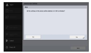
**3.** Confirm the message and press [Yes] to perform initialization, and the scanner will turn OFF.
