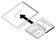
**3.** Load the document with the sealed end of the carrier sheet as the leading edge and the page you want to scan facing down.
