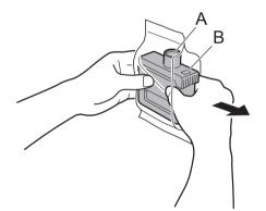
Never touch the ink holes (A) or metal contacts (B). Touching these parts may cause stains, damage the ink tank, and affect print quality.
