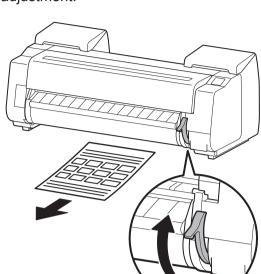
Load the next paper by referring to steps 2 to 5 on p.9. Print head adjustment uses 5 sheets of paper. Repeat steps 2 and 3 until the printing has finished.
