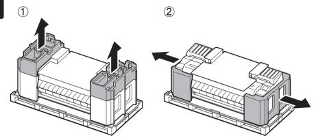
Remove all of the tape and other packaging material. Open the top cover (A) and output guide (B), and then remove the tape affixed to the roll holder.
