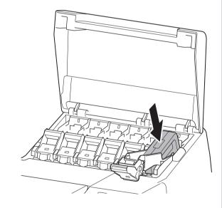
• An ink tank cannot be mounted in the holder if it is not oriented correctly for the
