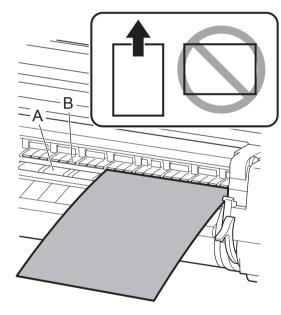
Load the paper aligned with the paper alignment lines (A) to ensure that the paper is not crooked, and align the leading edge of the paper with the front side of the line (B).
