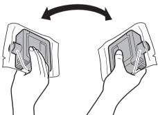
• Failure to shake the ink tanks may result in reduced print quality because ink ingredients have settled on the bottom of the tank.
