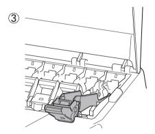
• Make sure the ink tank lock lever stays in the locked position.
