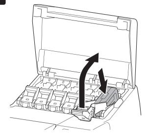
Firmly push down the handle part of the ink tank lock lever all the way in.
