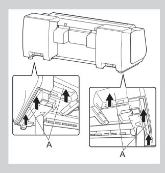
When standing up the printer or supporting the printer, hold the metal parts of the printer. If you hold a plastic part, the printer may become damaged.
