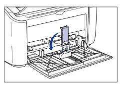
☐ Slide the rear paper guide to align the small paper guide with the paper.
