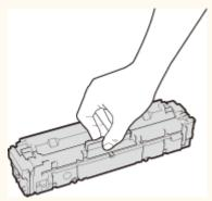
• To avoid scratching the surface (<sup>2</sup>) of the drum inside the machine or exposing it to light. Do not touch the electrical contacts (<sup>1</sup>) or the toner cartridge memory (<sup>2</sup>).
