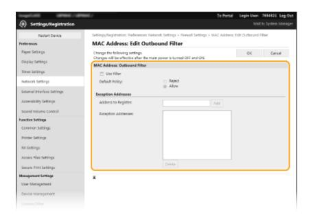
Select the [Use Filter] check box and click the [Reject] or [Allow] radio button for the [Default Policy].
