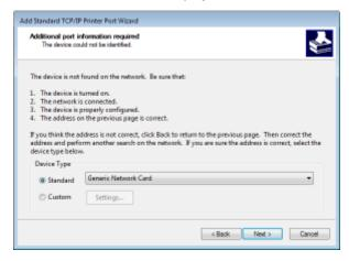
\*When you select the [Device Type], select [Canon Network Printing Device with P9100] under [Standard].
