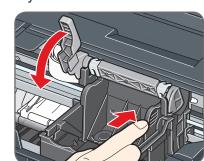
If the Top Cover is left open for more than 10 minutes, the Print Head Holder moves to the right. Close and reopen the Top Cover to return the Holder to the center
