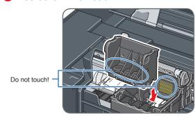
**6** Push the Print Head to hold it in place. and lower the Print Head Lock Lever carefully.
