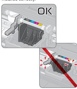
Be sure that the Print Head Lock Lever is pressed all the way down, and that the Print Head is locked firmly in place. If the Print Head is tilted forward, or the Print Head Lock Lever is pressed only halfway down, raise the Print Head Lock Lever and remove the Print head, and then reinstall the Print Head.
