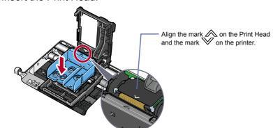
**5** Lower the Print Head Lock Lever carefully by pressing down the tabs on both ends until it clicks into place.
