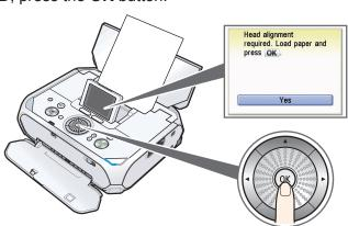
A pattern is printed and the Print Head is aligned automatically.
