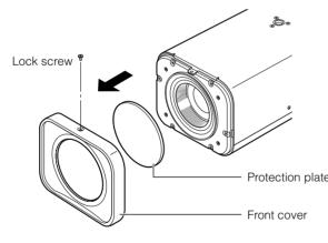
• When reattaching the protection plate, face the side with the cutout toward the lens.
