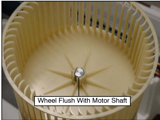
Figure 3-37 Evaporator Blower Wheel (Flush With End Of Motor Shaft)
