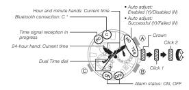
\* Hold down (B) for at least 2.5 seconds to establish a Bluetooth connection with a phone.
