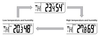
• To turn off temperature/humidity screen auto cycling, press the MAX/MIN button (8).
