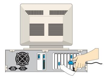
Check the serial port on the back of your PC. If the connector on the interface cable that comes with this kit does not match it, you will have to get an adaptor. Make sure you follow any instructions specified in your PC operating manual.
