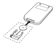
3 Replace the battery holder back into the remote controller.
