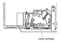
6 Pull up on the handle or ribbon to remove the lamp cartridge.
