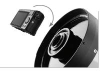
Once the camera is installed, you can adjust its orientation by slightly loosening the retaining ring. Loosen the ring no more than 1/8th turn, rotate the camera as desired, and retighten the ring.
