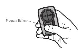
Test the remote control by pressing the button. If the product does not activate, repeat the programming steps or follow the alternative programming option.
