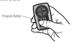
Test the Universal Remote Control by pressing the button. If the product does not activate, repeat the programming steps or follow the alternative programming option.
