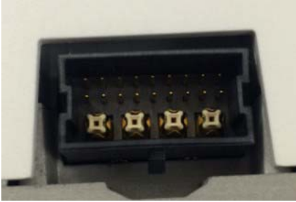
Figure 8 Smart Antenna Connector on 2802E Model
