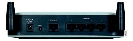
**POWER**—Connects the router to power, using the AC power cable.
