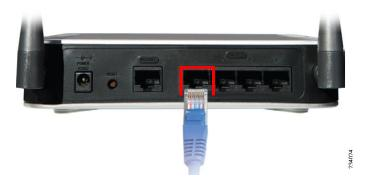
STEP 3 Repeat the previous step to connect more PCs, a switch, or other network devices to the router.
