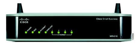
POWER—(Green) Shines steady when the router is powered on.
