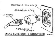
When the plug is inserted in a properly grounded receptacle box, it will protect the user from shock, should the tool insulation for any reason fail.
