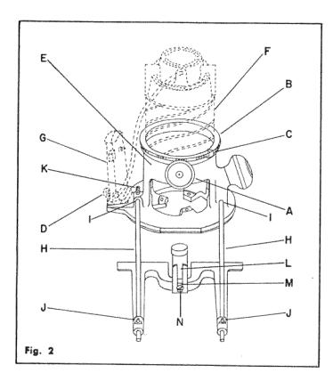
TO ASSEMBLE MOTOR UNIT TO BASE—Align slot in adjusting ring (B), Fig. 2 with slot in base (E). Insert motor unit (F) into base, with pin located in side of motor unit engaging slot in adjusting ring. Lower motor unit in slot until it bottoms. Then turn adjusting ring in a counterclockwise rotation to further lower motor unit. Attach motor unit handle by sliding onto base dovetail and tightening locking screw (D).
