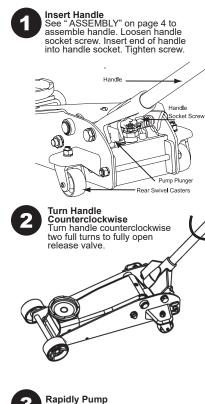
Rapidly pump the handle 6 - 8 times. Leave handle in down position to expose oil fill screw.
