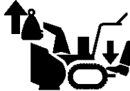
Weight Transfer Depress Pedal To Disengage
