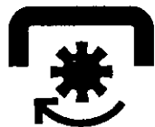
ATTACHMENT CLUTCH ENGAGED
