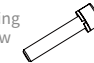
22 Hexagon socket head spring washer combination screw M5X12 x4 内六角圆柱头弹垫组合螺钉M5X12
