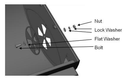
Attach the SIDE HANDLE to the right side of the CHARCOAL GRILL BODY using two (2) <sup>1</sup>/<sub>2</sub>" BOLTS and two (2) LOCK WASHERS as shown. From inside the GRILL BODY insert each BOLT through a LOCK WASHER and then through the GRILL BODY and then screw into the SIDE HANDLE. See below.
