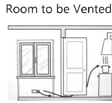
Room to be Vented Enlarging the ventilation slot between window and floor.
