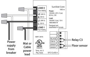
Sensor and relay connections are made to the terminal block by inserting the wires into the square openings and tightening the screws on the side.
