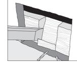
For retrofit installations. cut out drywall and chisel out the bottom plate to route wires to control.
