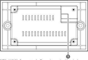
1 CAT5e/6/7 IN: Connect to the Transmitter unit with a single
