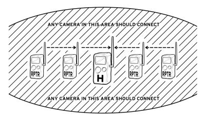
Use cameras or repeaters to create a Network Backbone. A Backbone allows cameras to be moved without breaking links to other remote cameras
