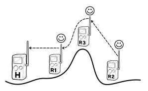
Use a repeater to extend range. A repeater is the best way to transmit over a hill or ridge.
