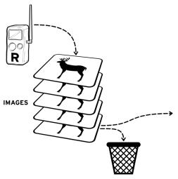
Remote cameras place images in an outbox to wait to be transmitted home. If the outbox is full the oldest image is deleted to make room for the newest. The size of the outbox is set by CL COUNT.
