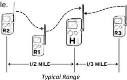
One CuddeLink equipped camera must be the HOME camera. HOME is the camera that collects images from the REMOTE cameras.
