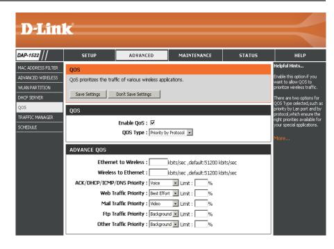
ACK/DHCP/ICMP/ Represents the priority value and bandwidth limit applied to ACK, DHCP, ICMP, and DNS for packet delivering.
