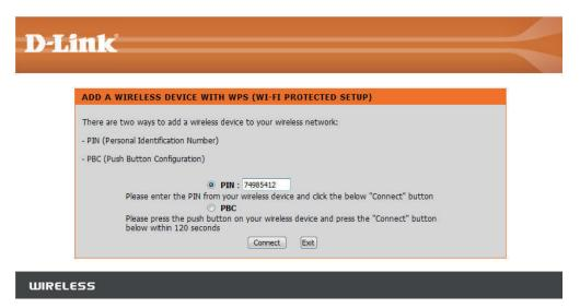
Start **WPS** on the wireless device you are adding to you wireless network to complete the setup.
