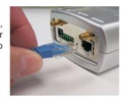
If you connect this camera directly to a PC, you will need a cross-over Ethernet cable. If you plug the camera into a hub or router, you will be able to use the cable included with your camera.
