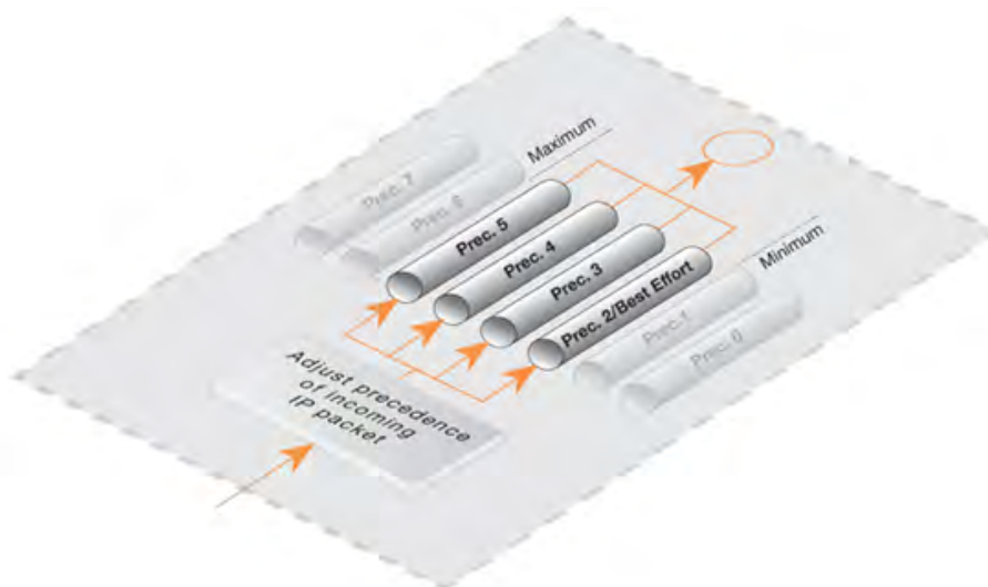
Figure 10.3. A Pipe defined with minimum precedence and maximum precedence.
