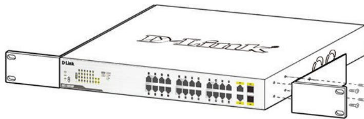
Figure 6 - Attaching the rack brackets
