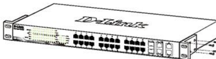
Figure 10 – Attach the mounting brackets to the Switch
