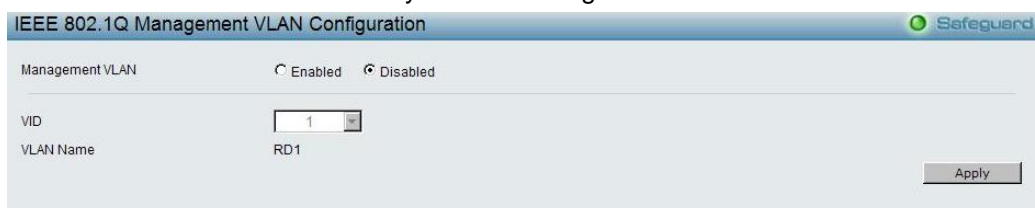
Figure 66 – Configuration > 802.1Q Management VLAN
