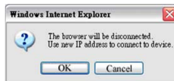
Figure 32 – Confirm the changes of IP address in Smart Wizard
