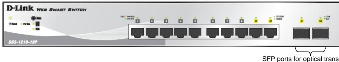
Figure 1 – DGS-1210-10P Front Panel
