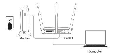
Plug the power adapter into your router and connect to an available power outlet or surge protector. If the Power LED does not light up, verify the power adapter is plugged in a working outlet or power strip.
