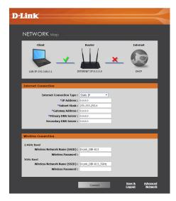
For both the 2.4GHz and 5GHz bands, create a name for your Wi-Fi Network and a password. Your wireless devices (i.e., tablets, smartphones, and laptops) will need to have this information entered to be able to connect to your wireless network. Click **Connect** at the bottom to continue.
