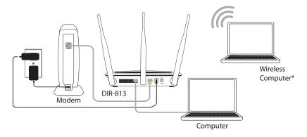
\* If you are connecting wirelessly, you may now connect to the router using the supplied Wi-Fi Configuration Card for the Wi-Fi network name (SSID) and Wi-Fi password.
