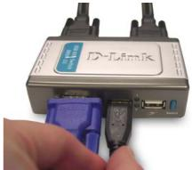
Attach your computer's USB mouse connector to the mouse port located on the DKVM-2U.
