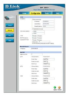
Select the **System** button under the **Configuration** tab to view the Print Server and Port names. If you change the names of the ports, please make note of them, as they will be needed during the Add Printer Wizard.
